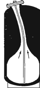
Condition 4 – System Pressure at 20 PSI Heated Water
