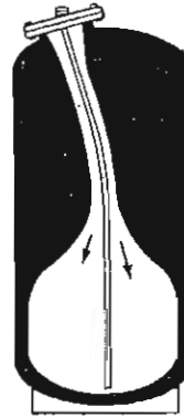
Condition 2 – System Pressure at 20 PSI Heated Water
