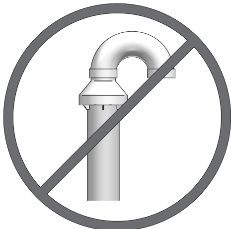
Figure 5-5 Do Not Install U-Bend to Rain Cap
