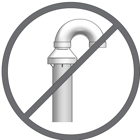
Figure 5-5 Do Not Install U-Bend to Rain Cap
