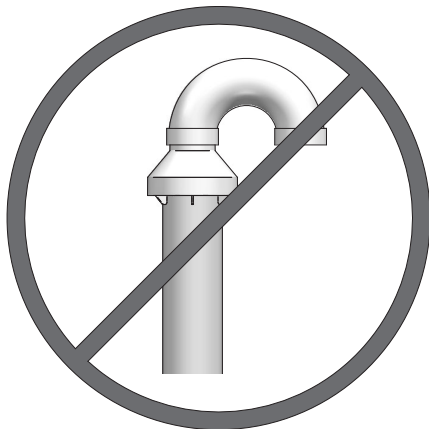
Figure 5-5 Do Not Install U-Bend to Rain Cap
