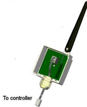
Figure 17: Location of the Wireless Receiver's telephone socket
