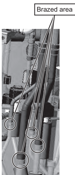
Removal of the rear heat exchanger on a high-efficiency model (Figure 18)
