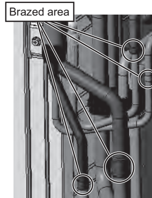
Removal of the left rear heat exchanger on a high-efficiency model (Figure 13)
