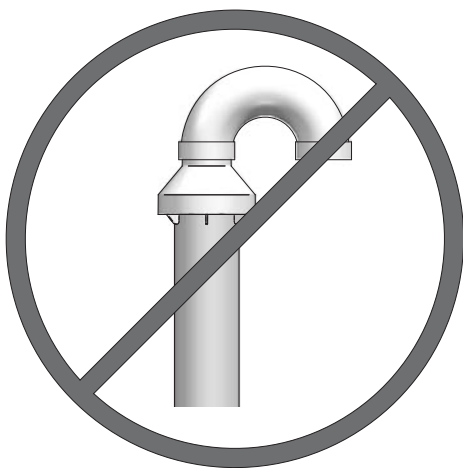
Figure 5-5 Do Not Install U-Bend to Rain Cap
