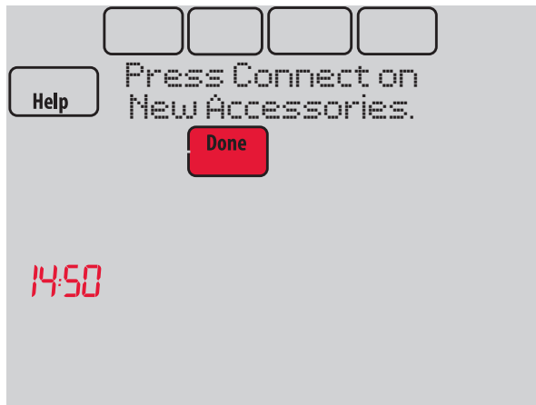
Fig. 43. Thermostat in listening mode.
