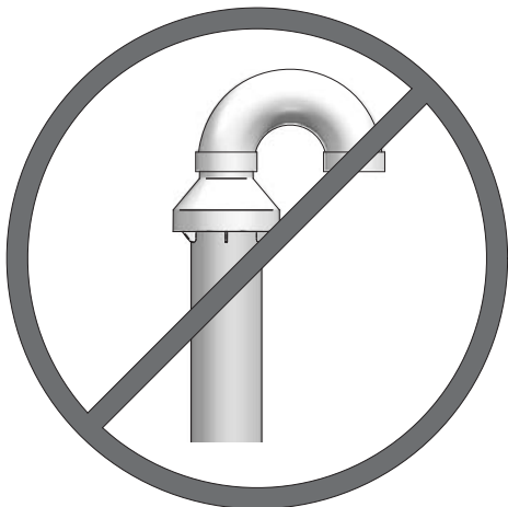
Figure 5-5 Do Not Install U-Bend to Rain Cap
