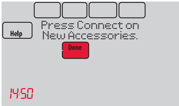
Fig. 35. Thermostat in listening mode.
